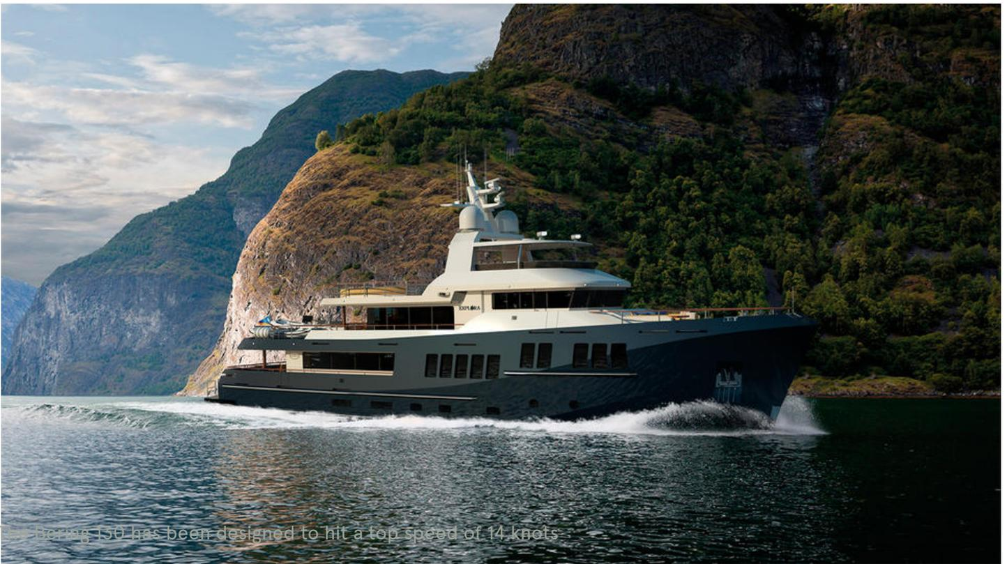
The yard adds that the tall bow profile provides the requisite stability needed to cross oceans and deal with heavy swells. This tri-deck explorer yacht features a Portuguese bridge and a maximum cruising range of 6,000 nautical miles, thanks to a 64,000 litre fuel capacity.
